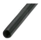
Protective hose, material: PA 6, UV-resistant: yes, flexible, degree of protection: IP68, color: black, flammability rating in acc. with UL 94: V0, inside diameter: 16.5 mm, Total length: 50 m
