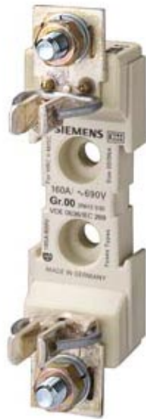
LV HRC FUSE BASE 690V(1000V) SINGLE-POLE, 160A, SIZE 00 PAD-TYPE TERMINAL, 95 SQMM
