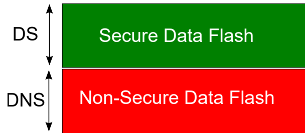
Figure 12-3. PIC32CM LS00/LS60 Data Flash Memory Mapping
