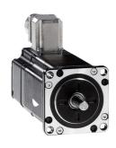
3-phase stepper motor - 1.02Nm - shaft Ø6.35mm -L=56mm - without brake -term box
