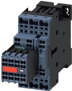
power contactor, AC-3e/AC-3, 12 A, 5.5 kW / 400 V, 3-pole, 24 V DC, with plugged-in diode combination, auxiliary contacts: 2 NO + 2 NC, spring-loaded terminal, size: S0, captive auxiliary switch
