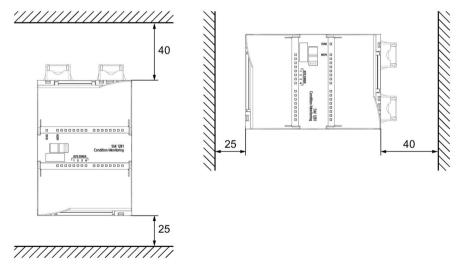
Figure 6-1 Minimum clearances with horizontal and vertical installation
