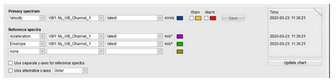
The current spectrum can only be displayed if the relevant IEPE channel has been configured and the spectrum has been calculated. Spectra from fingerprints, on the other hand, can be displayed irrespective of the current configuration and the current operating mode.
