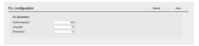
The center frequency is the start value of the speed calculation and should be close to the expected speed.
