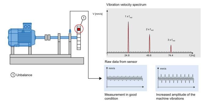
Figure 3-5 Example of a spectrum of vibration velocity (unbalance)
