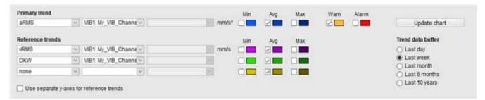
Up to 4 channel can be displayed at the same time. For each selected value, the minimum, maximum, and/or average value can be displayed. Up to 12 curves can be displayed in a fixed color scheme. For the "primary trend" you can additionally display the current warning and alarm limits specified by the S7.
