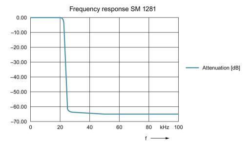
Figure 14-1 Filter characteristic curve for analog inputs of SM 1281
