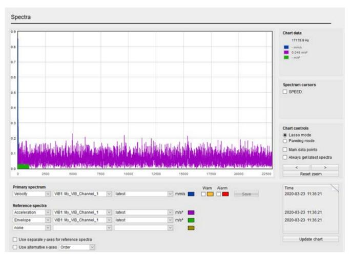
In the figure, the x axis shows the frequency and the y axis shows the amplitude. Alternatively, you can also set a scaling in "Revolutions per minute" or a non-unit "Order" (quotient of frequency and speed) for the x axis. If the background color is orange, the calculation was performed with values outside of the measuring range.
