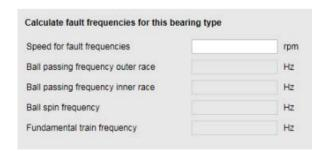
For direct entry of frequencies, you enter a speed as the reference value and the corresponding bearing fault frequencies for outer race, inner race, rolling element and cage.
