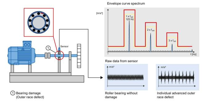
Figure 3-8 Example of envelope curve analysis
