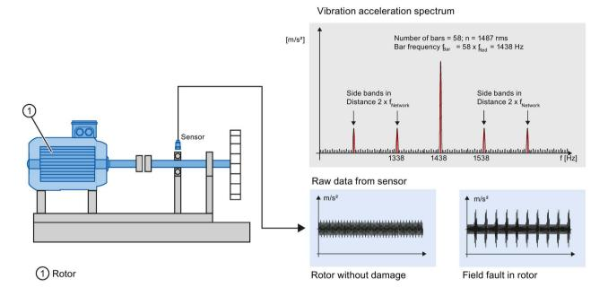
Figure 3-7 Example: Spectrum of the vibration acceleration (rotor field fault)
