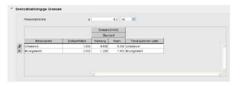
Figure 11-4 Speed-dependent limits
