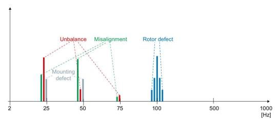
Figure 3-4 Overall spectrum of vibration velocity
