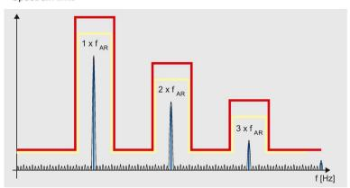
Figure 3-9 Spectrum limit band, speed-dependent
