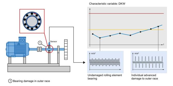
Figure 3-3 Example of a DKW characteristic value
