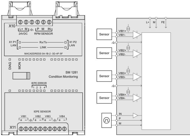
Figure 8-1 Connection diagram and block diagram
