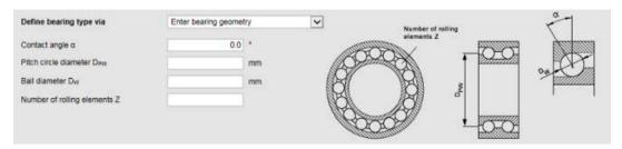
For entry of the bearing geometry, four geometric characteristic values are specified:
