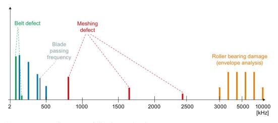
Figure 3-6 Overall spectrum of vibration acceleration
