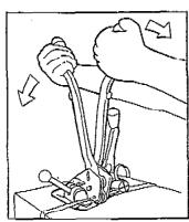
Open the two scaling levers. This will crimp the seal and cut the strap simultaneously.
