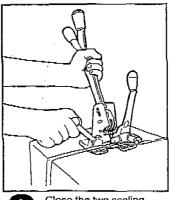
Close the two sealing levers and push back. Release clamp and remove tool.
