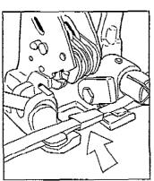
Apply seal, open end downwards, over the two superimposed parts of
