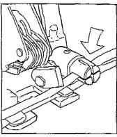
Take other end of strap, pass it under cutting blade and thread into cross slits of winch.
