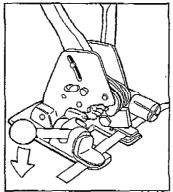
Lock loose end of strap into clamp after passing it under fixed base of cutter and winch roller.
