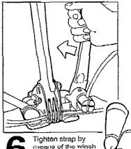
means of the winch lever until desired tension is obtained.
