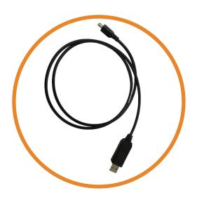
This is a custom cable, 1m long, which is used to connect the ITT and ITTU series of temperature transmitters to a compatible PC in order to configure the operating range and other parameters.
