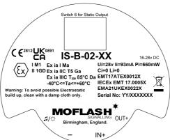
Year of Manufacture can be found as the first 2 digits of the serial number on the product label. These products have been tested by notified body **Element Materials Technology**, who are UKAS accredited to BS EN ISO/IEC 17025:2005 and ISO/IEC 17065:2012. It is also a Notified Body for the ATEX Directive, UKEX (UKCA), an IECEx Certification Body and an IECEx Testing Laboratory.
