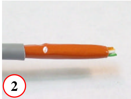
2 Remove 1" to 2" of cable jacket
