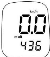
**IMPORTANT !** This instrument calculates altitude by using air pressure. It is therefore quite normal for the altitude to change when the air pressure changes. For this reason the instrument needs to be calibrated as often as possible.
