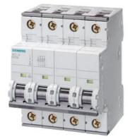
Miniature circuit breaker 400 V 25kA, 4-pole, 12.5 A, D=70 mm only magnetic tripping
