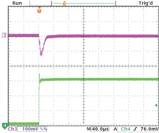
Step Load Transient Response (Vin=12V, Vout=3.3V, Cload=5x10µF
