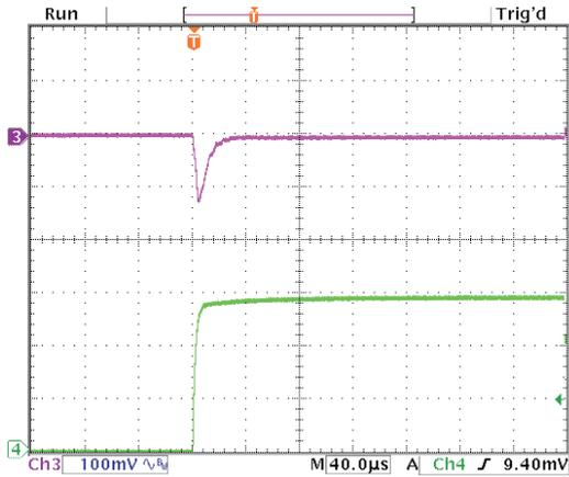
Step Load Transient Response (Vin=5.5V, Vout=3.3V, Cload=5x10µF
