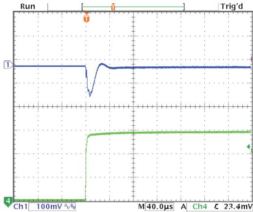
Step Load Transient Response (Vin=5.5V, Vout=3.3V, Cload=12x10µF X5R 0805 ceramic, total 120µF, Iout=3A to 0A) Top trace=Vout, Bottom trace=Iout
