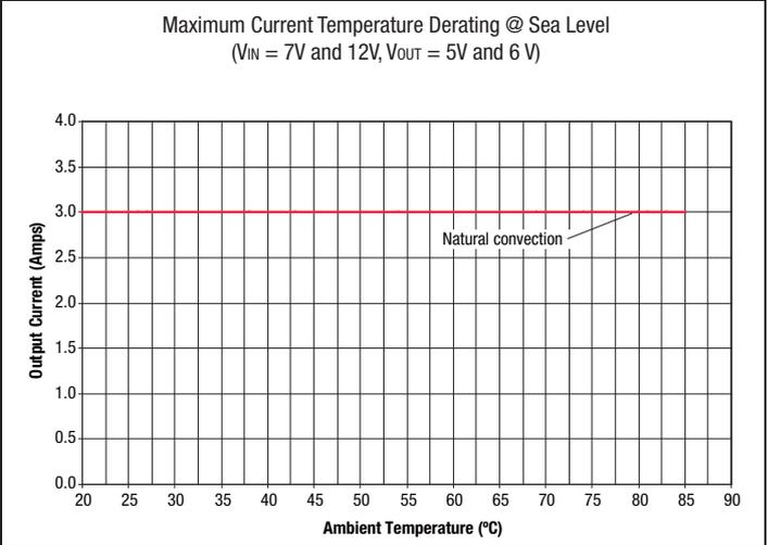
There is no derating for Vout = 0.591V. to 5.5V. at full load.
