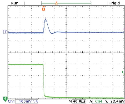
Step Load Transient Response (Vin=5.5V, Vout=3.3V, Cload=10x10µF X5R 0805 ceramic, plus 1x470µF, 7mΩ POSCAP, total 570µF, Iout=0A to 3A) Top trace=Vout, Bottom trace=Iout
