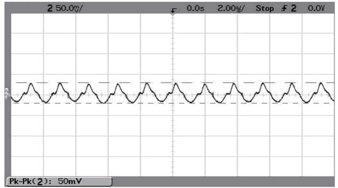
Step Load Transient Response (Vin=12V, Vout=5V, Cload=0, Iout=1.5A to 3A)
