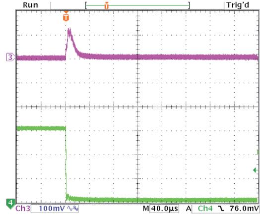
Step Load Transient Response (Vin=5.5V, Vout=3.3V, Cload=5x10µF
