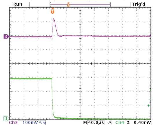
Step Load Transient Response (Vin=12V, Vout=1.8V, Cload=12x10µF
