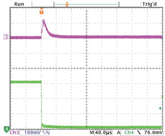
Step Load Transient Response (Vin=4.5V, Vout=1.8V, Cload=5x10µF
