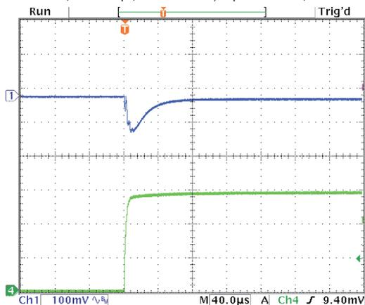
Step Load Transient Response (Vin=12V, Vout=1.8V, Cload=12x10µF
