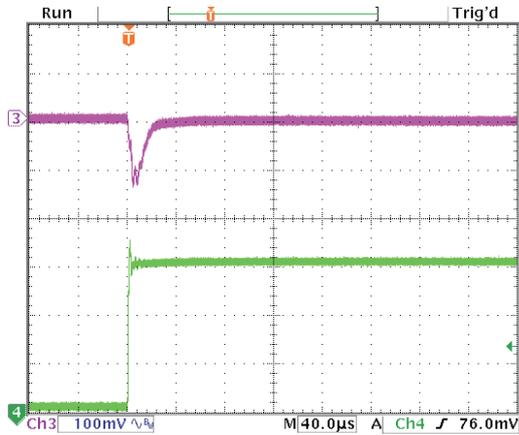
Step Load Transient Response (Vin=12V, Vout=1.8V, Cload=5x10µF
