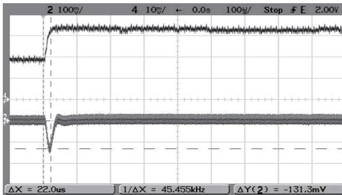
Step Load Transient Response (Vin=12V, Vout=5V, Cload=0, Iout=3A to 1.5A)
