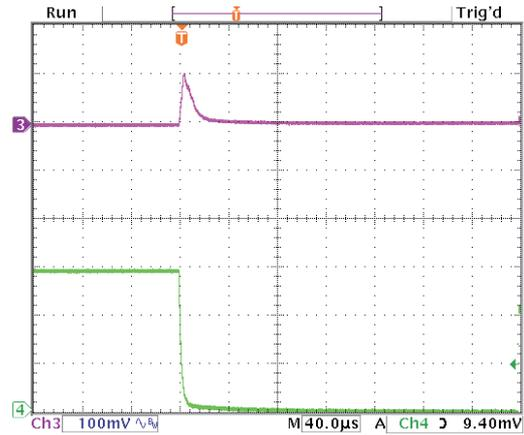
Step Load Transient Response (Vin=12V, Vout=3.3V, Cload=12x10µF
