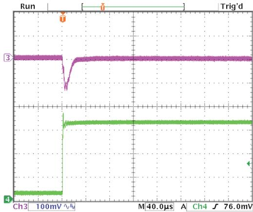
Step Load Transient Response (Vin=12V, Vout=5V, Cload=5x10µF X5R 0805 ceramic, total 50µF, Iout=3A to 0A) Top trace=Vout, Bottom trace=Iout
