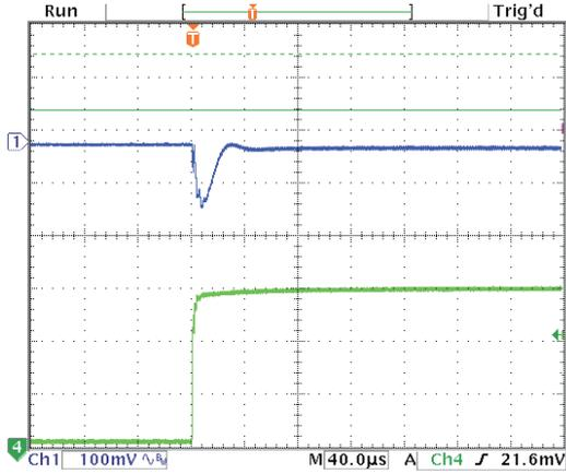
Step Load Transient Response (Vin=4.5V, Vout=1.8V, Cload=12x10µF X5R 0805 ceramic, total 120µF, Iout=3A to 0A) Top trace=Vout, Bottom trace=Iout
