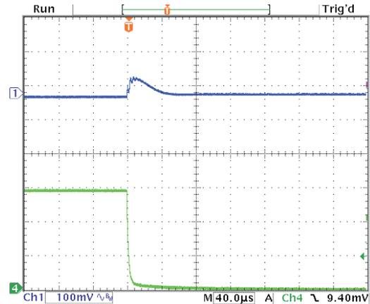
Step Load Transient Response (Vin=12V, Vout=3.3V, Cload=10x10µF X5R 0805 ceramic, plus 1x470µF, 7mΩ POSCAP, total 570µF, Iout=0A to 3A) Top trace=Vout, Bottom trace=Iout
