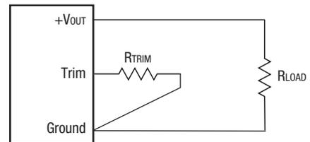
$$R_{TRIM} (k\Omega) = \frac{1.182}{V_{OUT} - 0.591}$$
