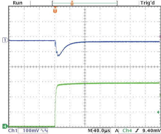
Step Load Transient Response (Vin=7.5V, Vout=5V, Cload=12x10µF X5R 0805 ceramic, total 120µF, Iout=3A to 0A) Top trace=Vout, Bottom trace=Iout
