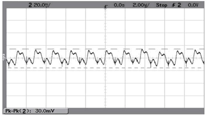
Step Load Transient Response (Vin=12V, Vout=2.5V, Cload=0, Iout=1.5A to 3A)
