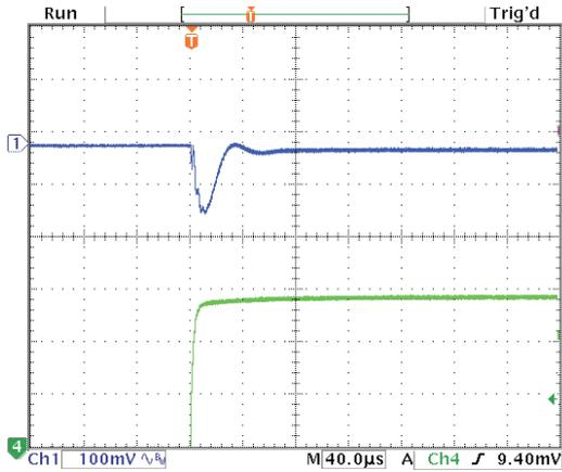
Step Load Transient Response (Vin=12V, Vout=3.3V, Cload=12x10µF
