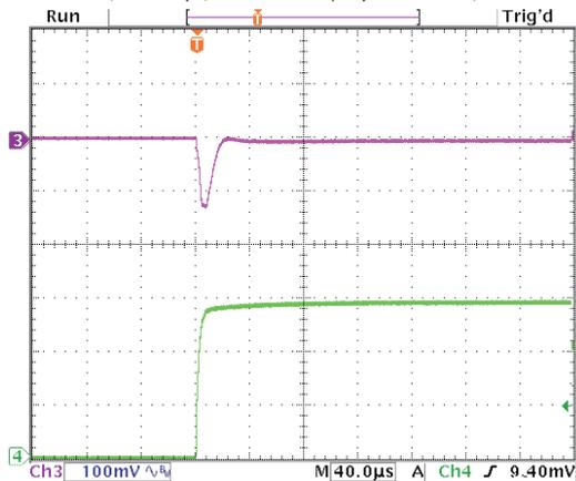
Step Load Transient Response (Vin=4.5V, Vout=1.8V, Cload=5x10µF
