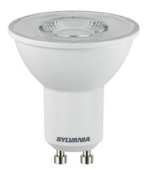
Compact, energy efficient and exceptional value LED GU10 lamp Same shape and size as halogen GU10 lamp Compact Cluster SMD technology enabling high efficiency with halogen look Reduced visible heat sink from the front Available in 110 degree beam angle High lumen efficacy 15,000 hours average rated life 3 years warranty
