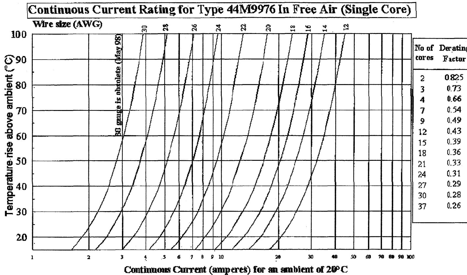
For ambients other than  $20^{\circ}\text{C}$ . divide the current by  $(234.5 + \text{ambient})/254.5$
