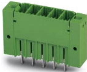
Header, Nominal current: 41 A, Rated voltage (III/2): 630 V, Number of positions: 4, Pitch: 7.62 mm, Color: green, Contact surface: Tin, Mounting: Soldering
