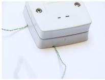
Attach the probe sensor to the object you wish to monitor using a TAPS adhesive pad or similar tape. Run the probe wire back to the TC Wall Port and fix the back panel to the wall using the slotted screw holes provided.
