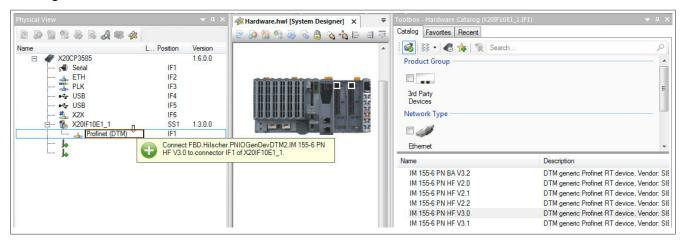
• Right-click on the IF interface and select "Device configuration" to open the configuration environment for the GSDML file.
