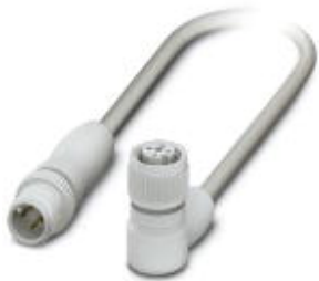
Sensor/Actuator cable, 4-position, PP-EPDM halogen-free, Gray RAL 7035, Plug straight M12, A-coded, on Socket angled M12, A-coded, Cable length: 3 m, Hygienic design, with plastic knurl
