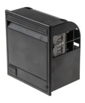
This RS Pro panel mount printer features a Seiko brand fixed head thermal line printer mechanism with a guillotine auto-cutter and anti-blockage design. It also has a large paper capacity. It has an electrical rating of 9-24VDC +/- 10%/2A. Interfaces featured are RS232/Parallel + USB/RS485
