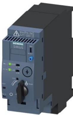
SIRIUS Compact load feeder DOL starter 690 V 110...240 V AC/DC 50...60 Hz 8...32 A IP20 Connection main circuit: plug-in, without terminals Connection auxiliary circuit: plug-in, without terminals
