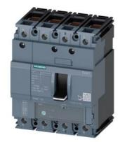
circuit breaker 3VA1 IEC frame 160 breaking capacity class N Icu=25kA @ 415V 4-pole, line protection TM220, ATFM, In=125A overload protection Ir=88A...125A short-circuit protection Ii=10 x In N conductor unprotected clamp connection
