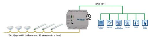
Integration of DALI drivers and sensors into a KNX installation.
