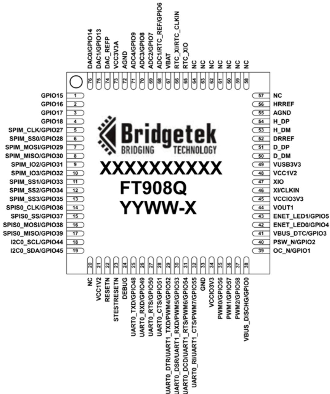
**Figure 3-4 - Pin Configuration FT908Q (top-down view)**
