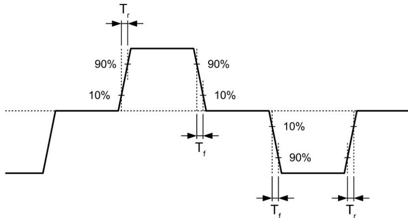
Figure 5-2 - 100Base-TX  $T_{r/f}$  Timing
