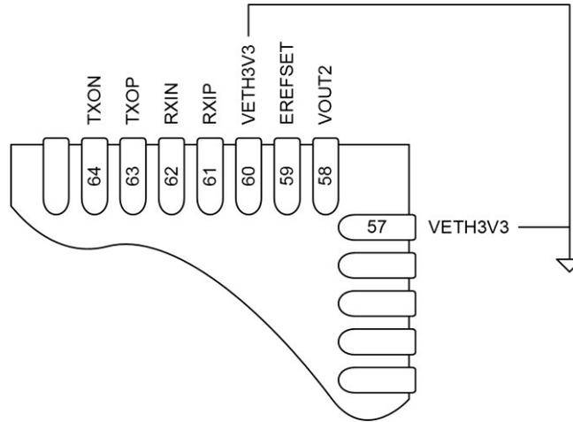
**Figure 6-8 - Unused Ethernet Connection (QFN)**
