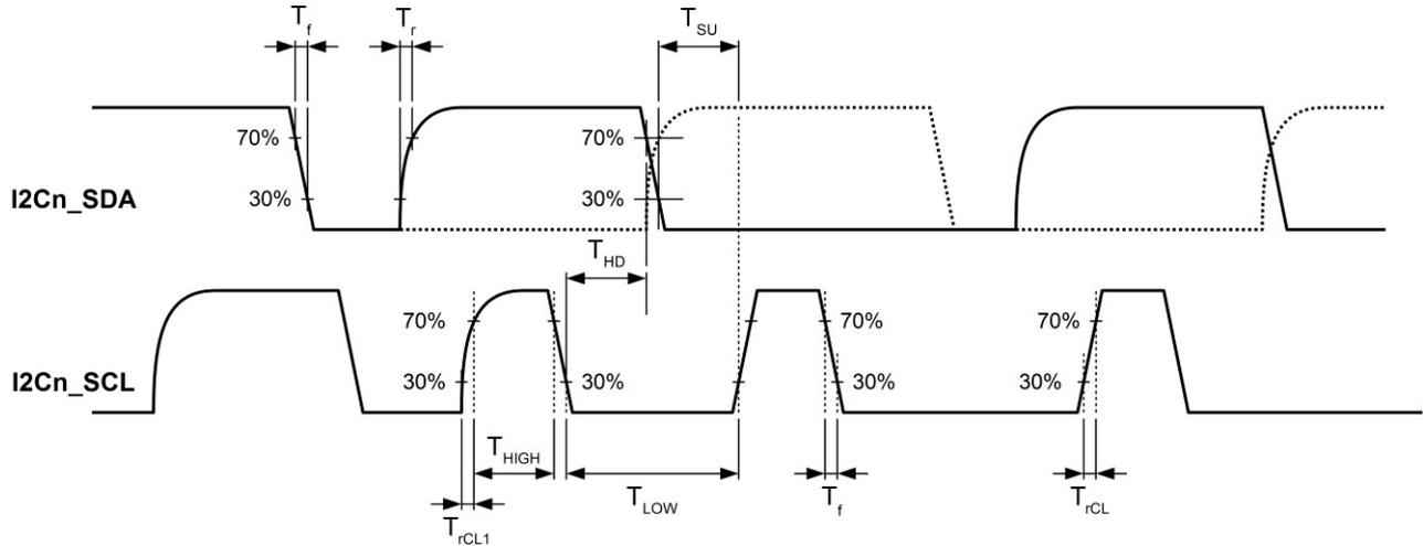
Figure 5-6 - Definition of I<sup>2</sup>C Timing HS mode
