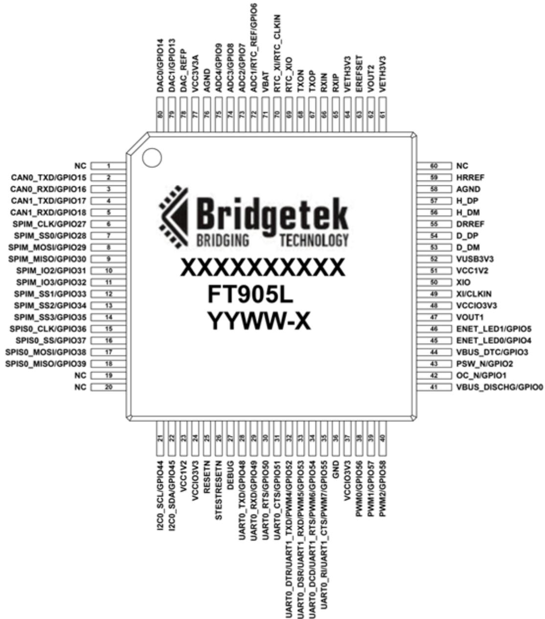
Figure 3-5 - Pin Configuration FT905L (top-down view)
