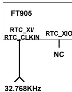
**Figure 6-4 - External 32.768 KHz clock input**
