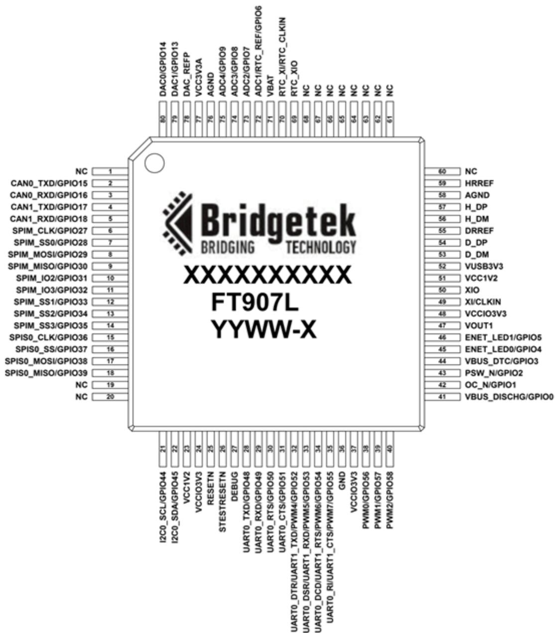
Figure 3-7 - Pin Configuration FT907L (top-down view)
