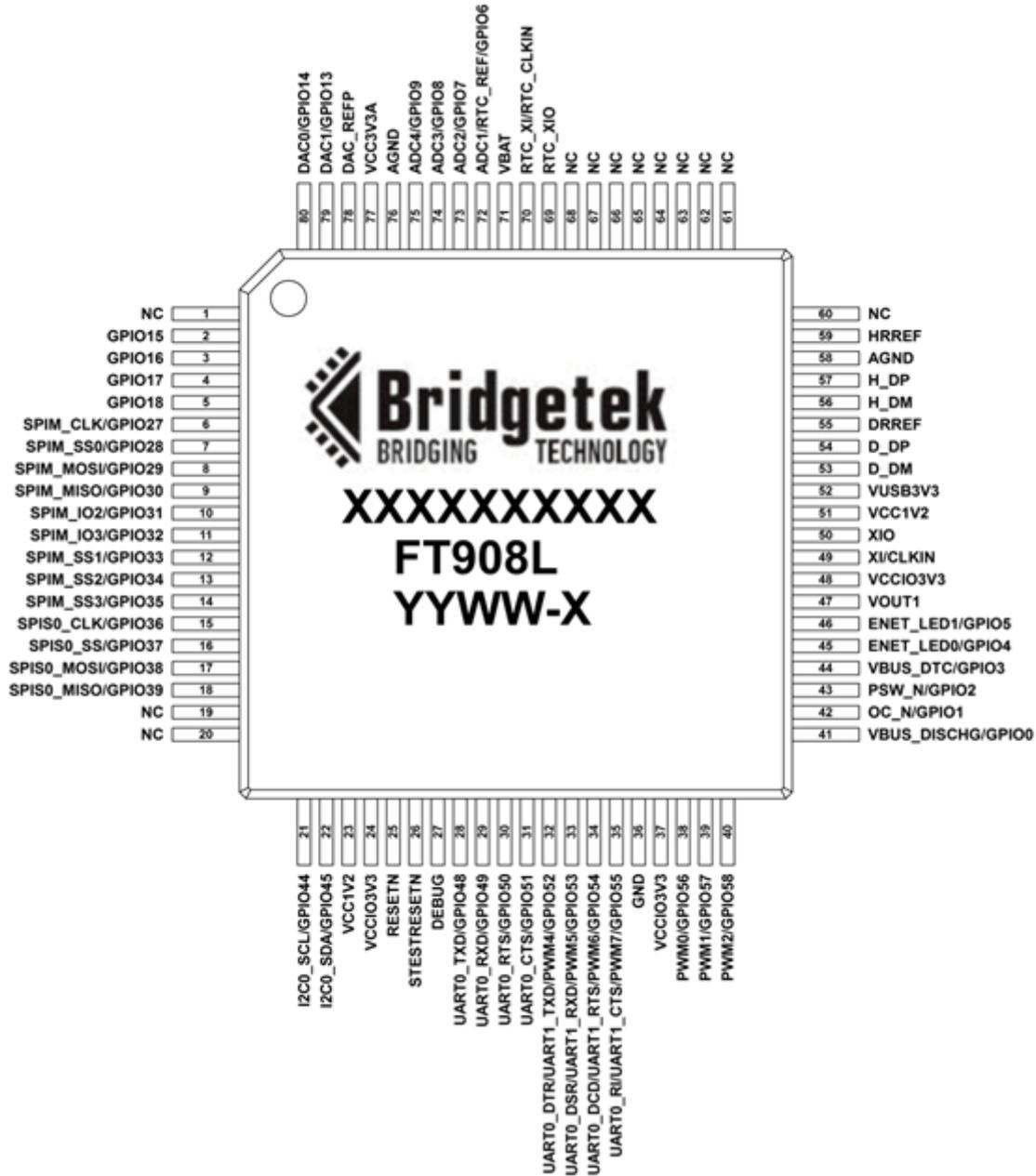
Figure 3-8 - Pin Configuration FT908L (top-down view)
