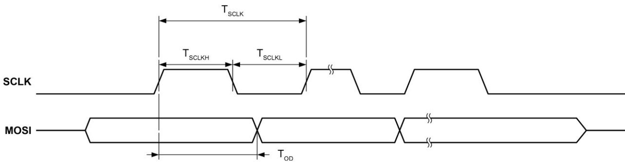
Figure 5-7 - Definition of SPI Master Timing Mode 0
