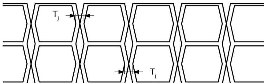
Figure 5-3 - 100Base-TX Jitter Timing
