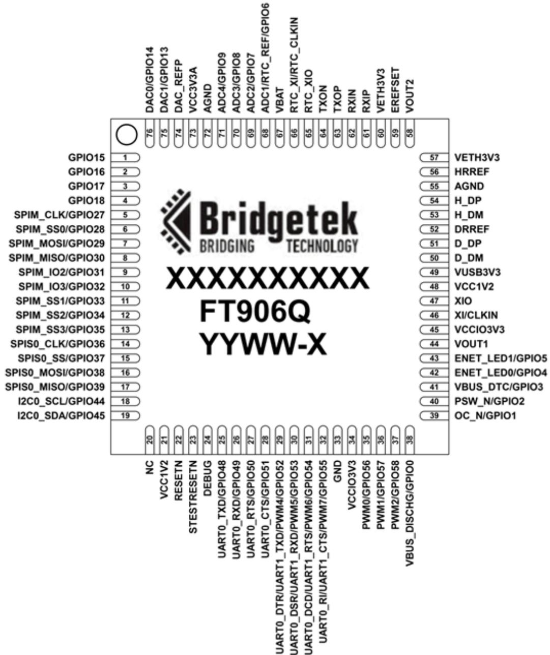
**Figure 3-2 - Pin Configuration FT906Q (top-down view)**
