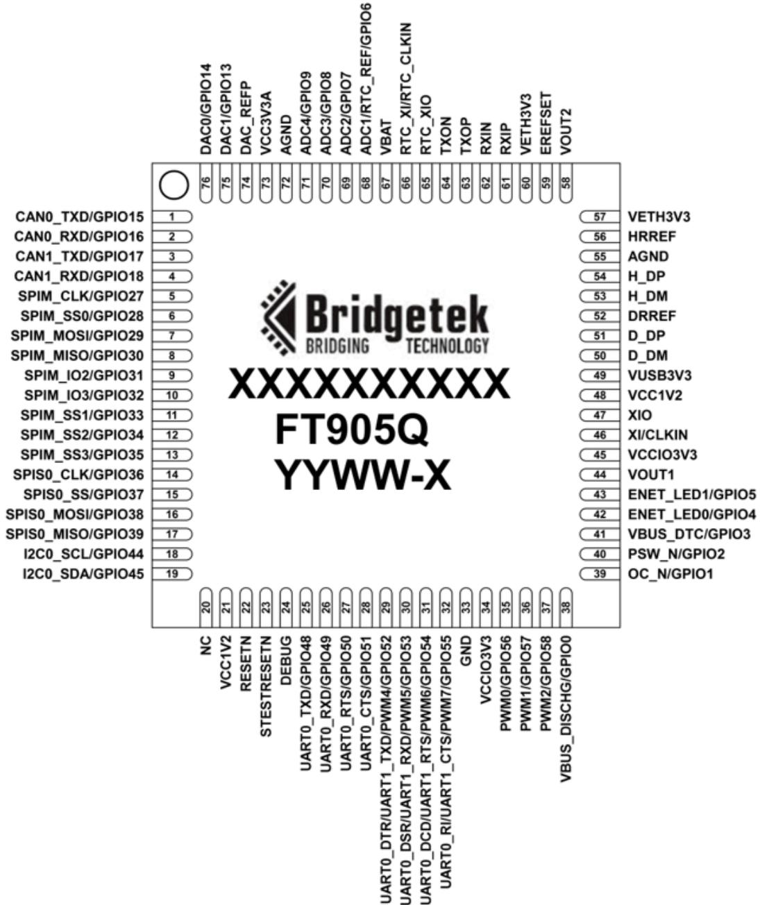
Figure 3-1 - Pin Configuration FT905Q (top-down view)
