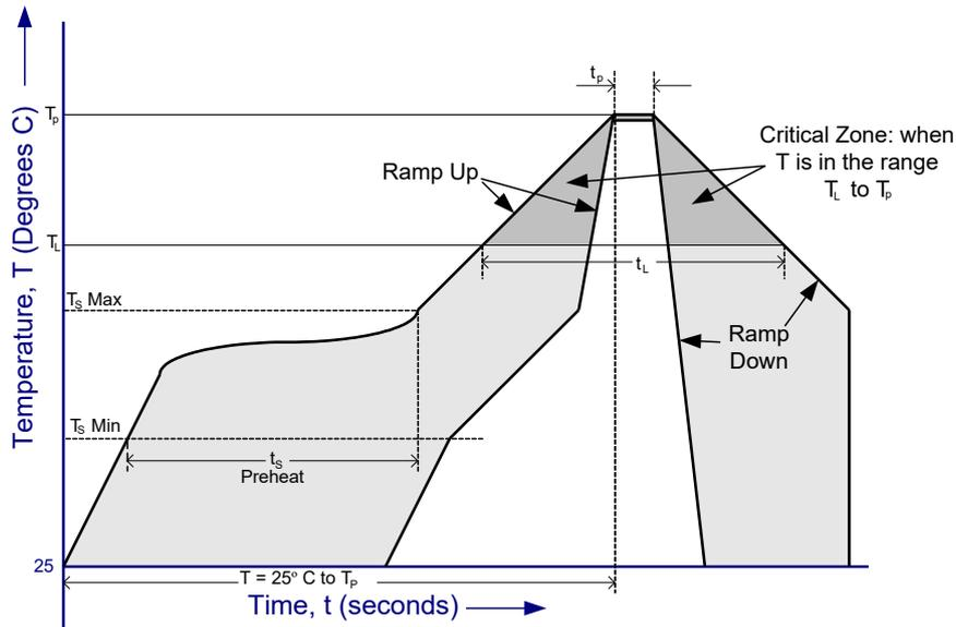
**Figure 7-5 - FT905 Solder Reflow Profile**
