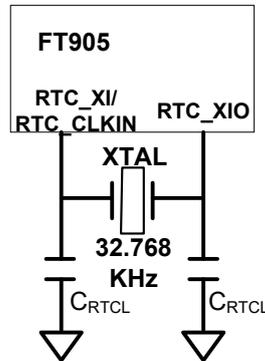
**Figure 6-3 - RTC 32.768 KHz oscillator connection**
