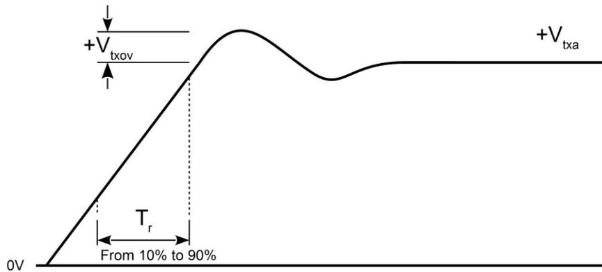
Figure 5-4 - 100Base-TX Transmission Waveform
