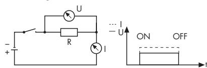
Voltage-current characteristic when switching a relay coil (illus. 2).
