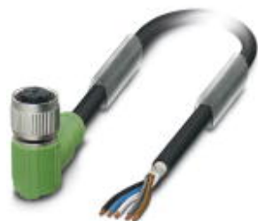
Sensor/Actuator cable, 5-position, PUR halogen-free, black-gray RAL 7021, shielded, free cable end, on Socket angled M12 SPEEDCON, A-coded, Cable length: 1.5 m
