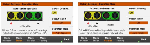
Figure 3. Auto-series and parallel operation together doubles the output voltage/current
