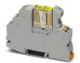
Pre-assembled relay module with Push-in connection, consisting of: relay base, safety relay with force-guided contacts in accordance with DIN EN 50205, plug-in display/interference suppression module, and retaining bracket, contact type: 2 changeover contacts, input voltage: 24 V DC
