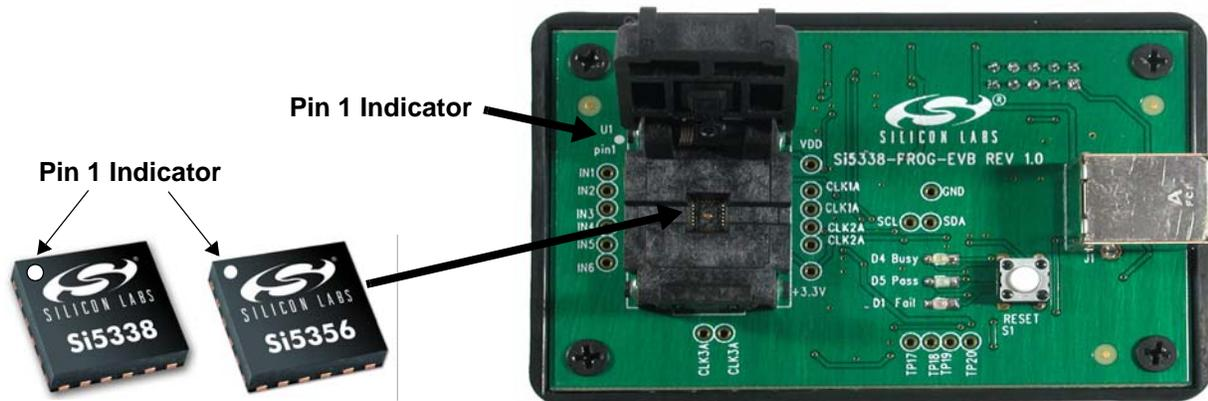
3. Once the device is properly loaded, close the lid. Ensure that the lid is fully closed and in the locked position. Some tension is normal when closing the lid. This ensures proper contact with the device.
