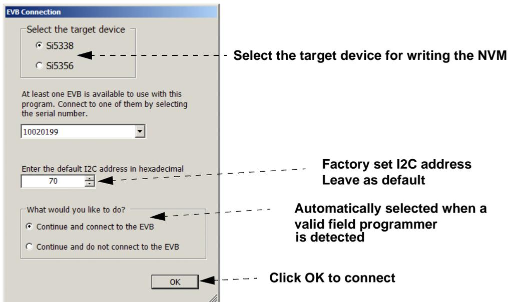
3. All devices shipped from the factory are pre-programmed with an I<sup>2</sup>C address of 0x70. The field programmer software will automatically use this I<sup>2</sup>C address when communicating with a device loaded into the socket. If the device has a different I<sup>2</sup>C address, enter its new address in the box provided.
