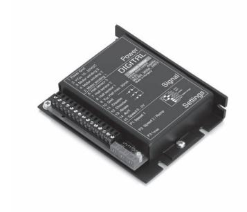
The DEC 50/5 (Digital EC Controller) is a 1-quadrant amplifier for controlling EC motors with Hall sensors with a maximum output of 250 watts.
