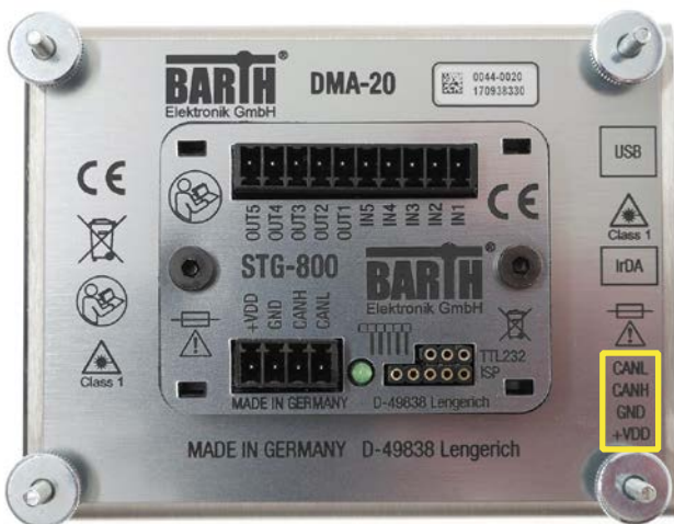
Connector (marked yellow): Power supply and CAN terminals
