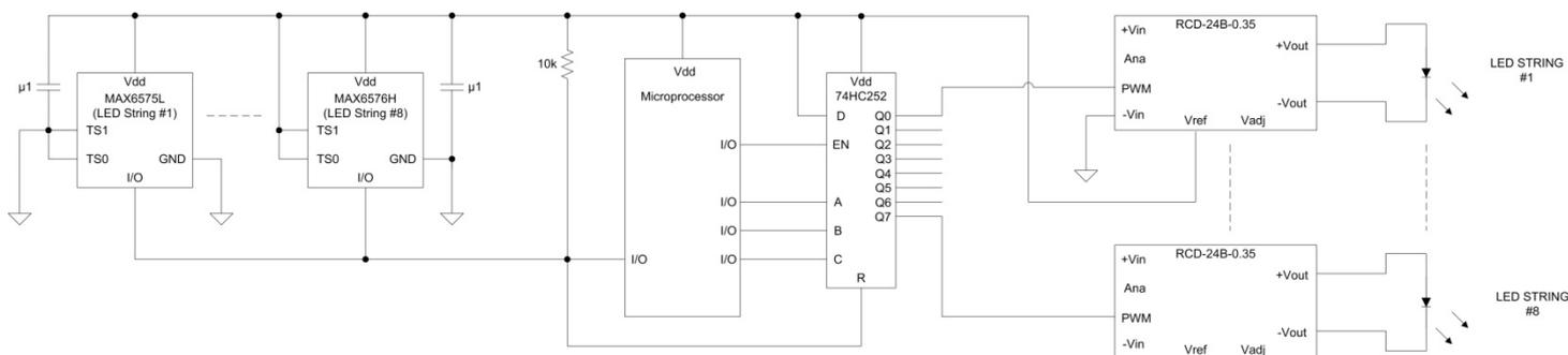
**Figure 5: Microprocessor-based PWM controller for up to eight LED drivers**
