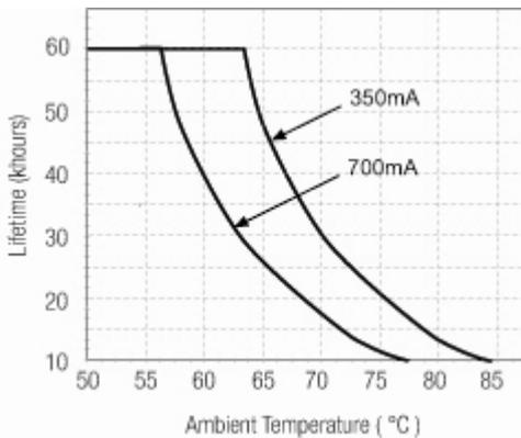
**Figure 1a: Effect of ambient temperature on lifetime derating curve**
