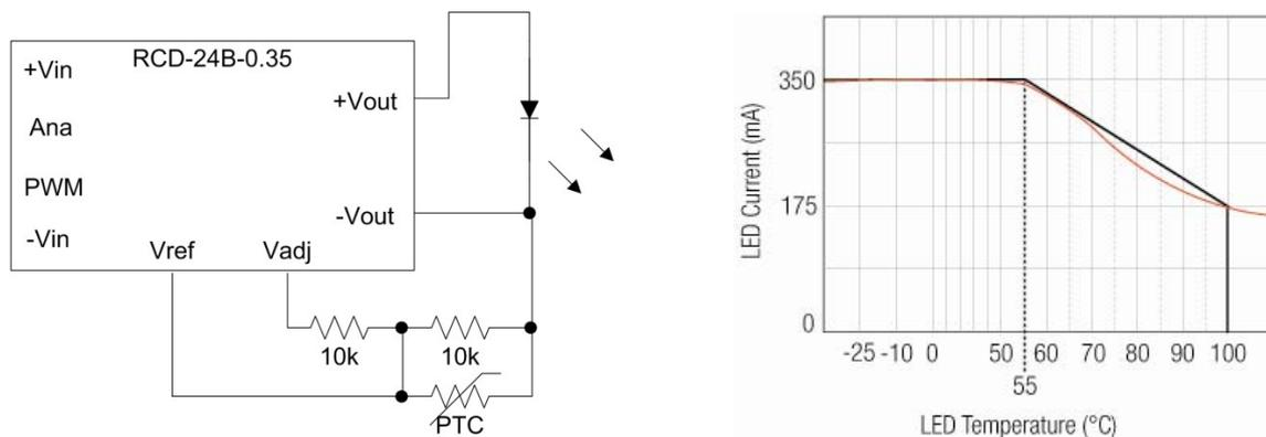
Figure 3: PTC Thermistor circuit and resulting LED derating curve (red line)
