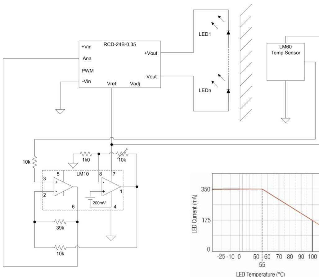
Figure 4: Analogue over-temperature circuit and resulting LED derating curve (red line)
