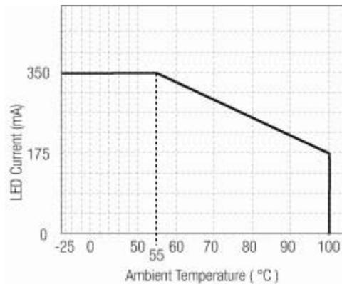
**Figure 1b: Typical LED temperature derating curve**
