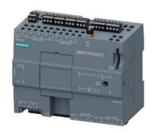
SIMATIC RTU3011C compact low-power RTU; battery or solar-operated; connection external power supply 10.8 V to 28.8 V DC; connection of external modem; GNSS; connection to TeleControl Server Basic; loadable protocols: DNP3, IEC 60870-5-104, SINAUT ST7 or MQTT; onboard I/Os: 8 DI, 8 DO, 4 AI; FTP client; configuration/diagnostics via web server; time synchronization; email; SD card slot. GNSS national approvals to be considered!
