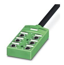
Sensor/actuator box, Connection method: M12-SPEEDCONsocket, Number of slots: 6, Number of positions: 5, Slot assignment: Double, Status indication: Yes, pnp; Master cable connection: Fixed connection 180°, PUR/PVC, Cable length: 5 m, Shielding: No
