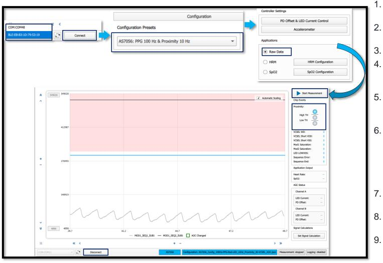
Fig. 14: Selection of PPG with proximity configuration file
