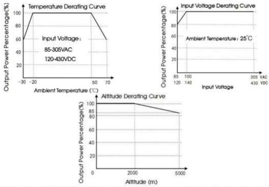
Note: U With an input voltage between 85-100VAC and a DC input between 120-140VDC the output power must be derated as per the temperature derating curves;
