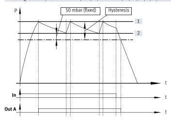
If the desired threshold value [1] for the vacuum is reached, vacuum generation is automatically switched off. A check valve prevents a decrease of the vacuum. Nonetheless, leakage (e.g. due to rough workpiece surfaces) will slowly reduce the vacuum. If the vacuum drops below the threshold value [2], vacuum generation is automatically switched on. Vacuum is generated until the set threshold value [1] is reached again.
