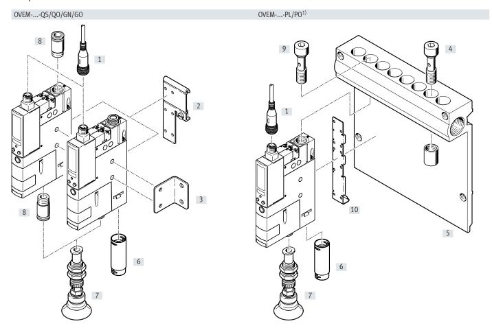
$1) \qquad \text{Hollow bolt [9] and mounting bracket [10] are included in the scope of delivery for the OVEM-...-PL/PO.} \\$
