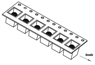
Figure 20. Unit Orientation from reel
