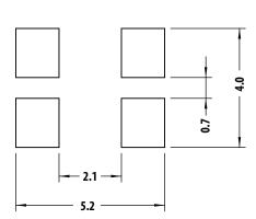
Note: Recommended stencil thickness is 0.1524mm (6 mils) minimum and above
