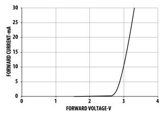
Figure 7. Forward Current vs Forward Voltage
