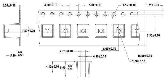
Figure 18. Carrier Tape Dimension
