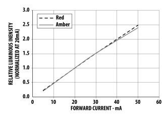
Figure 3. Relative Intensity vs Forward Current
