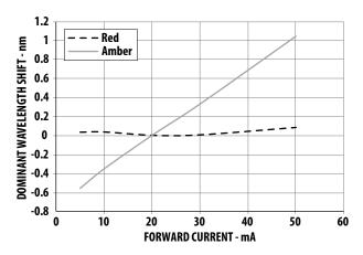
Figure 5. Relative Dominant Wavelength Shift vs Forward Current
