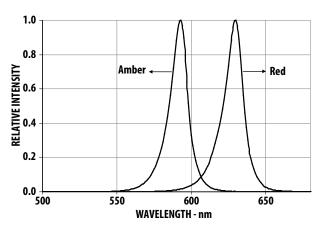
Figure 1. Relative Intensity vs Wavelength
