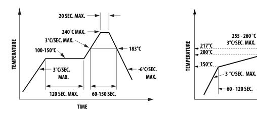
Figure 16. Recommended Leaded Reflow Soldering Profile
