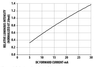
Figure 8. Relative Intensity vs Forward Current
