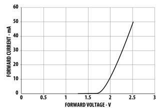
Figure 2. Forward Current vs Forward Voltage
