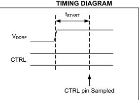
If the POR settings are satisfactory for the application, a microcontroller output pin can be freed by placing a weak pull-up or pull-down resistor on the CTRL pin. Only the DATA pin needs to be connected to an I/O pin.
