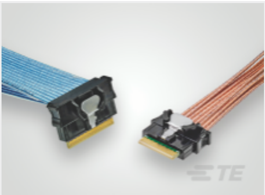
TE製品番号:2821750-1 SLIVER C/A, 50P, STR TO STR 25GHZ 100OHM
