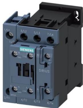
contactor AC-1, 40 A, 400 V / 40 °C, 4-pole, 110 V AC, 50 Hz / 120 V, 60 Hz, auxiliary contacts: 1 NO + 1 NC, screw terminal, size: S0
