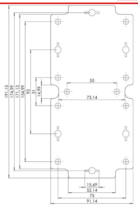
Dashed line shows outline of the mounting boss under PCB board Recommended mounting holes diameter ø2,6mm All dimensions are given within +/-0,5mm tolerance
