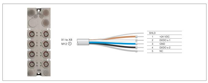
① X67CA0A41.xxxx: M12 sensor cable, straight X67CA0A51.xxxx: M12 sensor cable, angled
