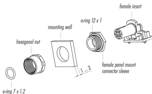
Product description **M12 Female angled panel mount connector, Contacts: 4, shieldable, THR, IP68, UL 2238, M12x1.0, Front mounting, for PCB assembly**
