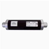
Fuse-link, medium voltage, 71 A, AC 17.5 kV, 3", 76 x 292 mm, back-up, DIN, with striker
