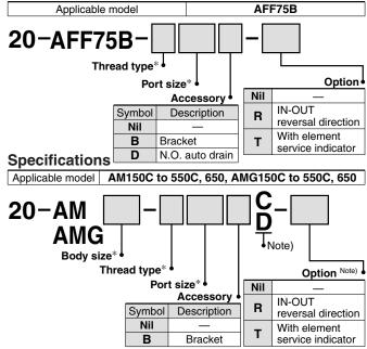
Note) "20-" is only applicable with N.C. auto drain (C) or N.O. auto drain (D). Drain cock and drain guide are copper-free, fluorine-free as standard
