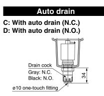
Combination of D: With auto drain (N.O.) and H: For medium air pressure
