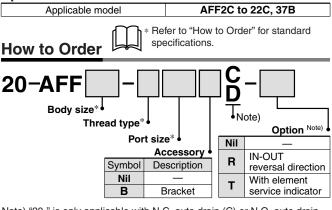
Note) "20-" is only applicable with N.C. auto drain (C) or N.O. auto drain (D). Drain cock and drain guide are copper-free, fluorine-free as standard.
