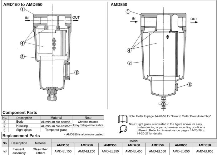
\* Element assembly: With gasket and O-ring
