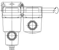
2. Do not apply torsional moment or bending moment (except the product's own weight) to the bracket. It may damage the bracket. Support external piping separately.
