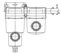
3. Inflexible piping such as steel piping tends to be affected by spread of excessive moment load or vibration from the piping side. Lay flexible tubing between the steel pipe and the product to prevent such effects.
