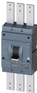
circuit breaker 3VA2 IEC Frame 1250 breaking capacity class H Icu=85 kA @ 415 V 3-pole line protection ETU350 LSI In=1250 A overload protection Ir=500 A ...1250 A short-circuit protection Isd=15... 10 X Ir li=10 x In circuit breaker with straight bus connectors extended
