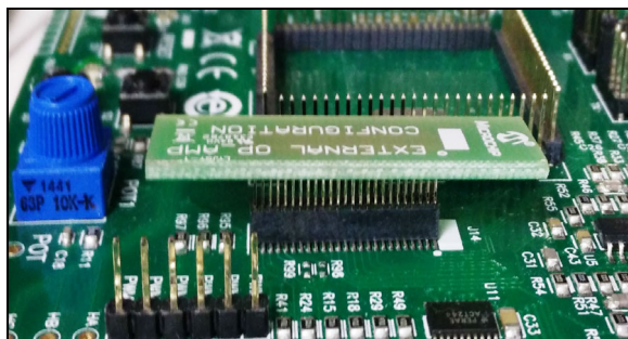
FIGURE 1: EXTERNAL OP AMP CONFIGURATION BOARD
