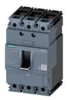
circuit breaker 3VA1 IEC frame 160 breaking capacity class S Icu=36kA @ 415V 3-pole, line protection TM210, FTFM, In=20A overload protection Ir=20A fixed short-circuit protection Ii=16 x In nut keeper kit
