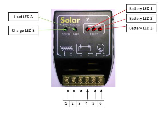
**Battery LED 1, 2 & 3** on, battery fully charged, **1 & 2** on, battery normal/healthy, **1** on only, battery low.
